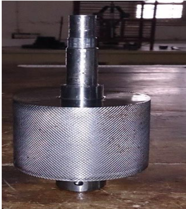
Figure 12: Shaft with crossed knurling
