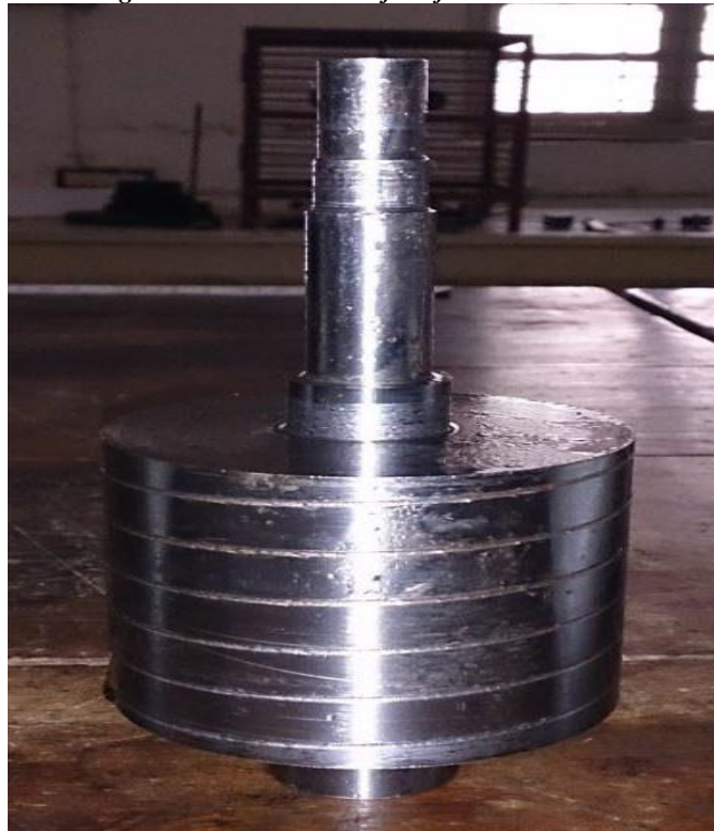
Figure 16: Shaft with a tool mark
