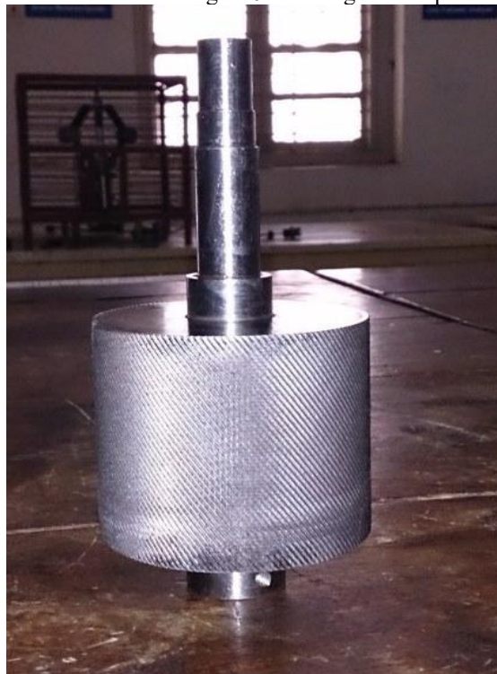
Figure 8: Shaft with straight knurling
